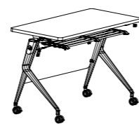
培训桌高配合置物架和挡板 Training Desk With Panel & Supporter (Top End) W1200*D500/550/600*H770 W1400*D500/550/600*H770 W1500*D500/550/600*H770 W1600*D500/550/600*H770
